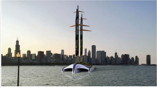
A conceptual image of Blue Technology's Liberty (pictured), a trimaran vessel that would not require a ballast-water treatment system. Credit: Blue Technology
